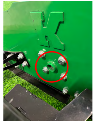
Lubricate the coupling, otherwise the bearing will cut and the coupling will break. (right and left side)
