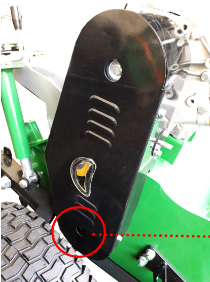
Lubricate the coupling, otherwise the bearing will cut and the coupling will break. (right and left side)
